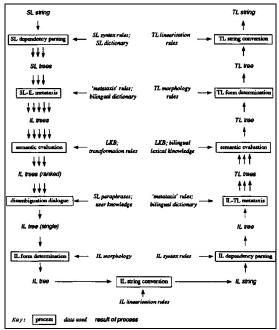
Figure 4: The overall design of the DLT system
