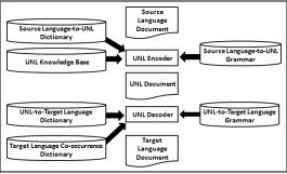
Figure 15: The overall architecture of the UNL system
